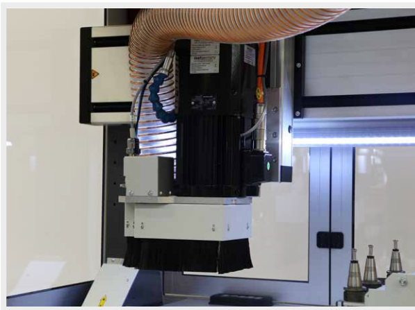
Option: suction device equipped with suction head
